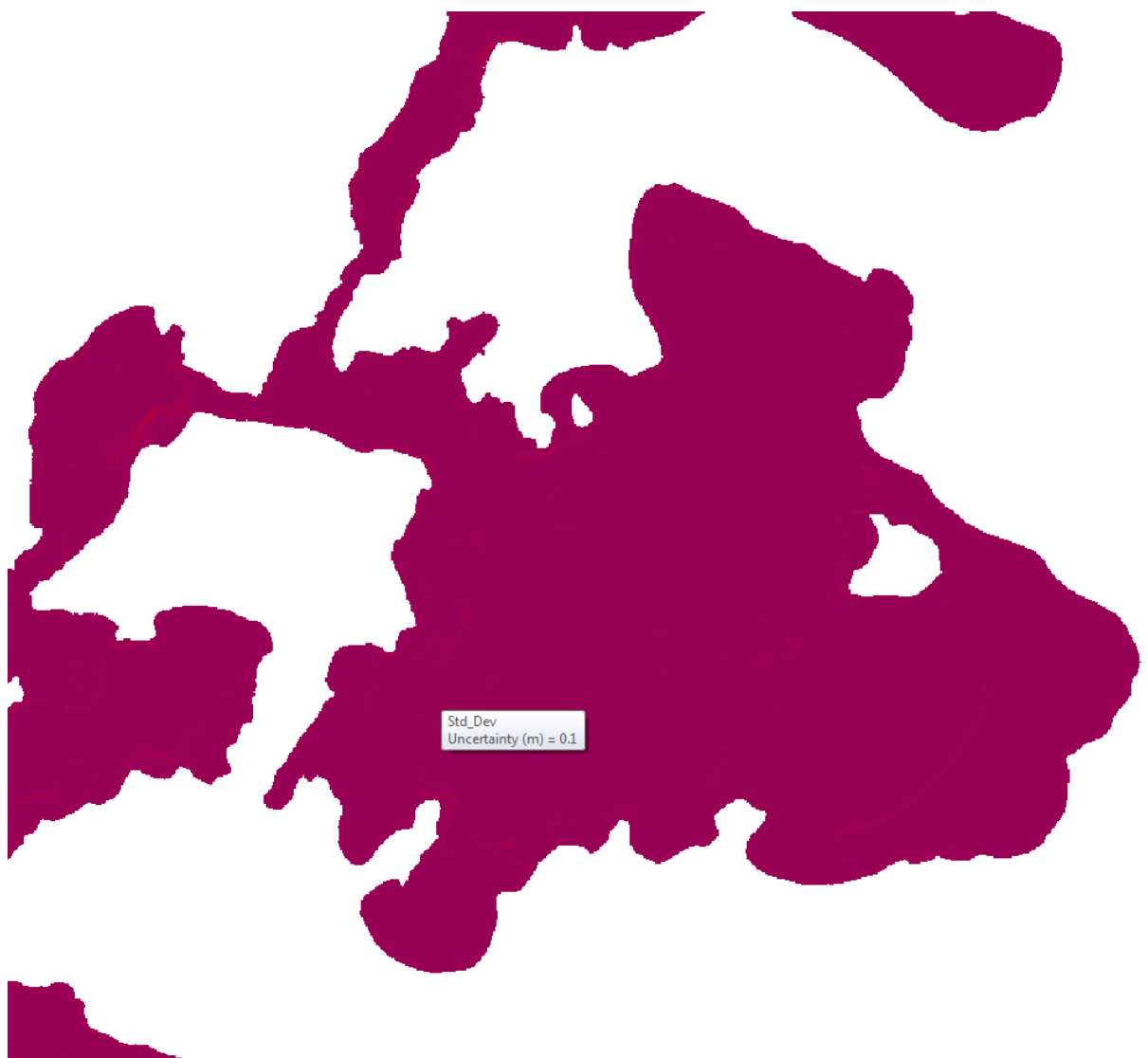
Fig. 9. Shows the area of uncertainty for hydrographic chart-0208 by using standard deviation. Each cell has an uncertainty value that tells about the spread in the data. Some cells have been observed where Std_Dev = 0. This is quite simply where only one sounding is included, or two soundings with the same depth value.
