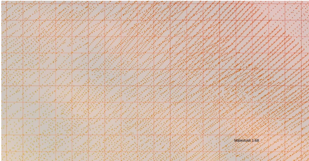
Fig. 5: If we are generating an S-102 terrain model, we first specify a resolution that is in accordance with the source data/soundings. The resolution will vary with the depth and echo sounder used during collection. In the illustration above a 2-metre resolution is specified, and every route in the network is 2 \times 2 metres.
